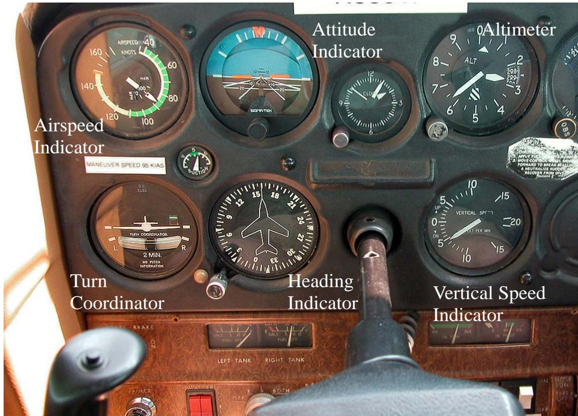
**Airspeed Indicator** – It provides information about the speed of the aircraft relative to the air in knots.
