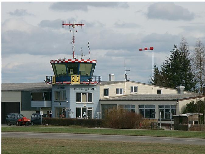
*Wind sock* A vital indicator to the pilot of wind strength and direction. When the sock is horizontal, the wind speed is approximately 20-25 knots.
